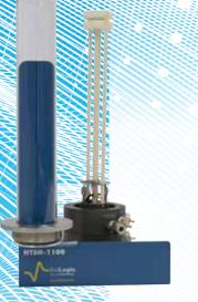
High Temperature Sample Holder (HTSH-1100) is a test fixture dedicated to characterization of electrical properties of solid materials using the parallel plate capacitor method over the temperature range between the room temperature and 1100 °C. HTSH-1100 can also be used for heat treatment in controlled atmospheres.
